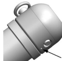
A note for racers: If your tech inspector wants you to safety wire these (most will not) then you simply need to orient the pins so that the pull on the pin is both clockwise and down (so that it acts to both tighten the bolt and pull the pin into the puck)
