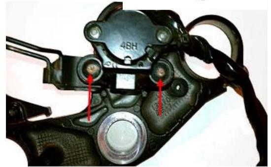
4. Reinstall the top triple clamp. **NOTE:** to reinstall the key switch at a later date, remove the studs from the underside of the clamp and replace them with regular bolts. To make these connections secure, you can use button head allen bolts for installation and then drill the hex out so that it is round.
